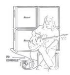
The low level, high impedance signal from the guitar pick-up is translated by the AR-133 into the high-level, low impedance balanced signal required by the front-of-house console.
