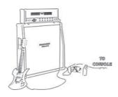
Taking a feed from the amplifier output allows the post-amplifier, post EQ/effects signal to be fed to the console, meaning that a particular effect/amp sound can be sent to the mix.
